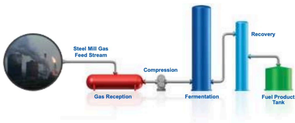
Figure 2: Production chain for the production of ethanol from BOF gas, as an example of gas fermentation (source: LanzaTech)
