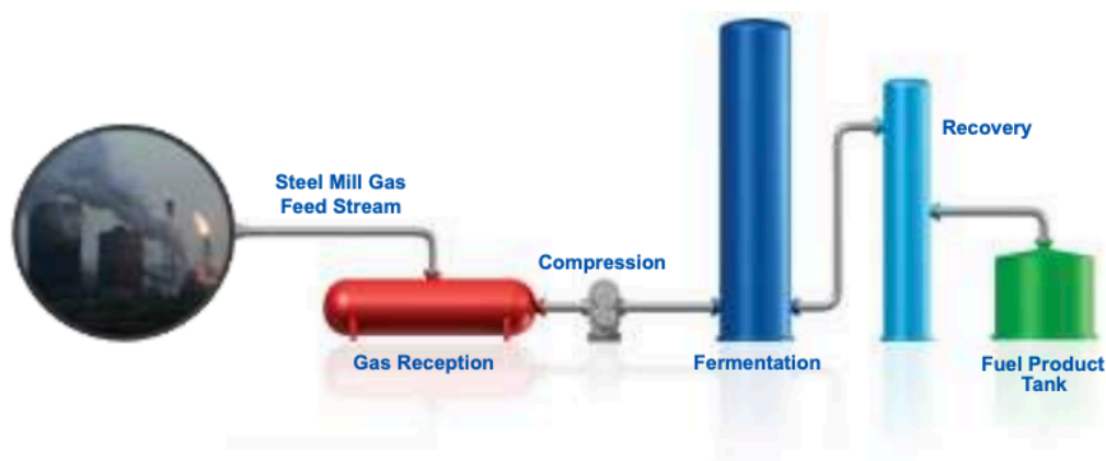
Figure 2: Production chain for the production of ethanol from industrial off-gas (source: LanzaTech)
